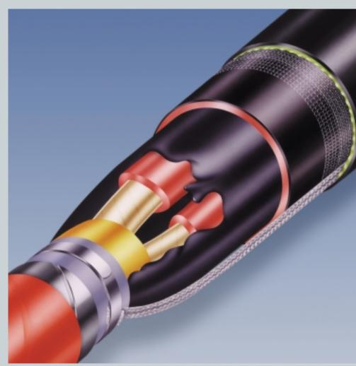
The EFSJ is versatile. It is factoryengineered for use on belted or screened, three-core, paper insulated, MI and MIND cables. Each basic joint kit can accomodate several cable sizes, so only four kits are required for the range of cross sections from 16 to 300 mm<sup>2</sup>.
