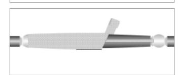
4. The copper earth braid and steel armour wrap are installed.
