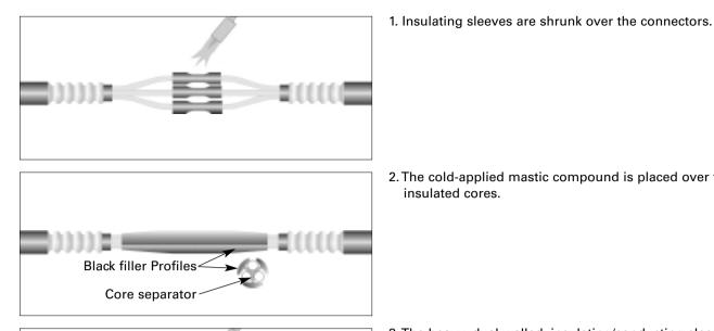
2. The cold-applied mastic compound is placed over the insulated cores.
