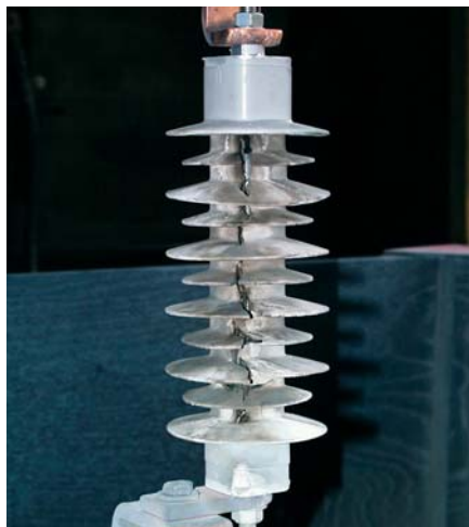
Safe short circuit failure
