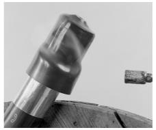
Simply heat the cap until it has shrunk tightly over the cable end.
