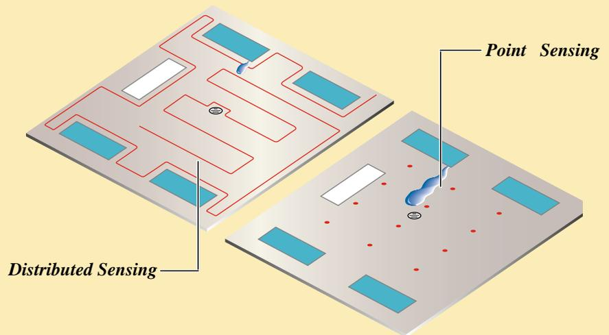
*A TraceTek locating system detects the leak at its source, signals the alarm, and displays the exact distance to the leak. By referring to a map of the system layout (supplied as part of the TraceTek system), you can quickly locate the leak source.*
