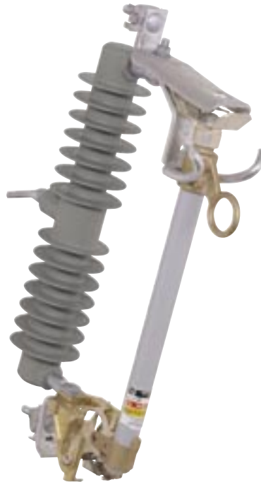
Catalog Number 89052R10-P-D▲ Ultra-Heavy-Duty Overhead—Pole-Top Style, rated 25 kV▼ nominal, 27 kV maxi- imum, 150 kV BIL, 100 amperes con- tinuous, 12,000 amperes interrupting RMS asymmetrical (16,000 amperes single-shot), 17 inches (432 mm) mini- imum leakage distance to ground.◆
