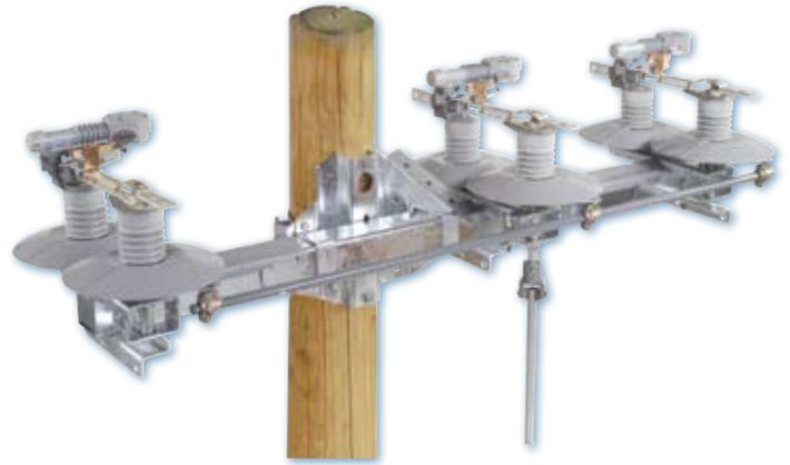
**Interrupters** provide no-external-arc interruption. Interrupter housings are molded from glass-reinforced polyester and include a two-part urethane coating for protection against weathering and ultraviolet radiation
